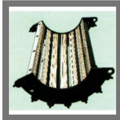
Blow Room Pinned Beater Segment
