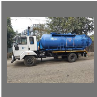
Suction Cum Sewer Jetting Machine
