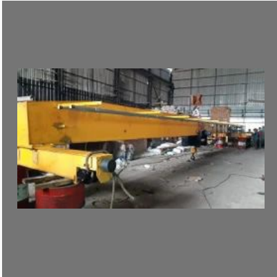
Crane End Carriages
