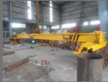
10Ton Single Girder EOT Crane
