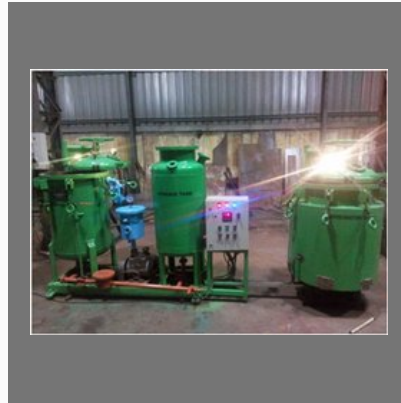
Vacuum Pressure Impregnation Plant
