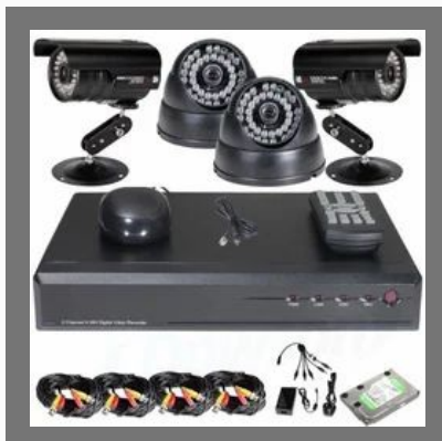
CCTV DVR System
