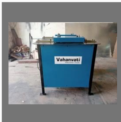
Duct Forming Machine
