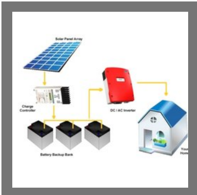
Off Grid Solar Power Plant
