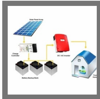
Off Grid Solar Power Plant
