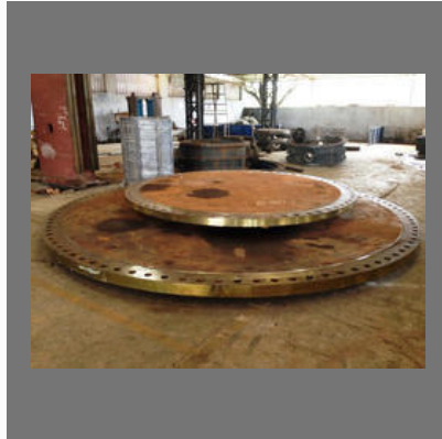
Blind Flange Machining Job Work
