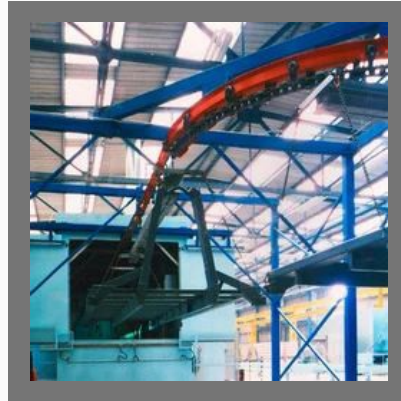
Overhead Chain Conveyor
