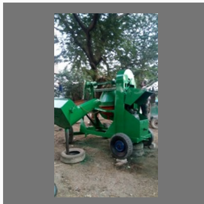
Diesel Cement Mixture
