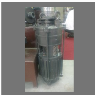
Vertical Water Pump
