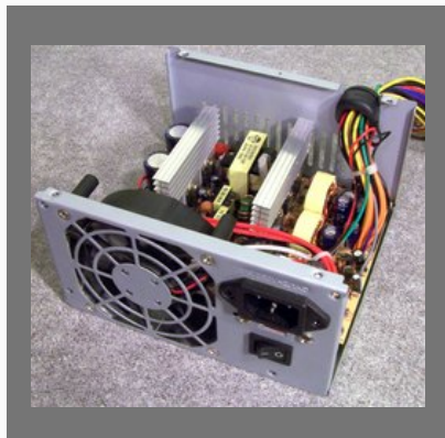
5A CCTV Power Supply
