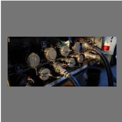
Bottom Loading Tank Truck Equipment
