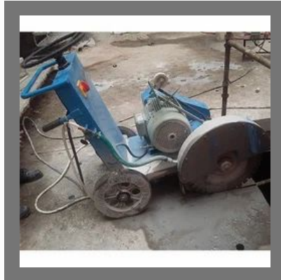
Concrete Road Cutting Machine
