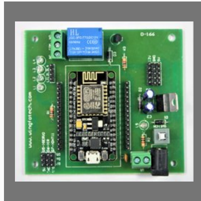
IOT(Internet Of Thing) Development Board with NodeMCU
