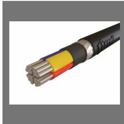
4 Core X 35 Sq.mm ALU XLPE ARMOURED CABLE
