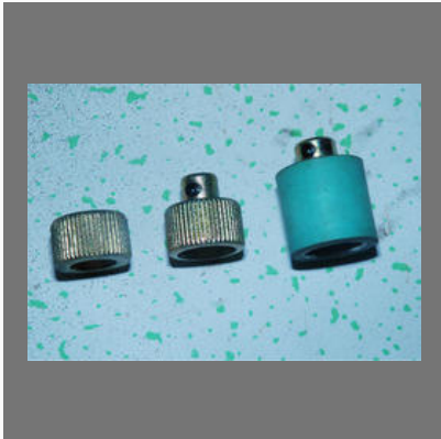
Agarbathi / Incense Machine Metal Roller and PVC Roller
