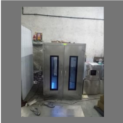
Clean Room Hatch Box
